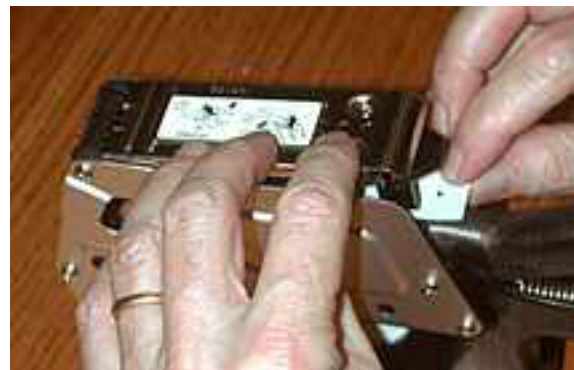
Close the bottom cover. (Label waste is dispensed between the handles.) Your price-marker is now loaded and ready for action!
